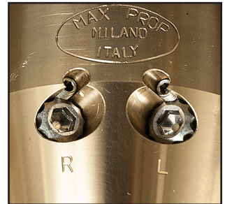
Fig.4 - Close up of the Left and Right pitch adjustment bolts.
